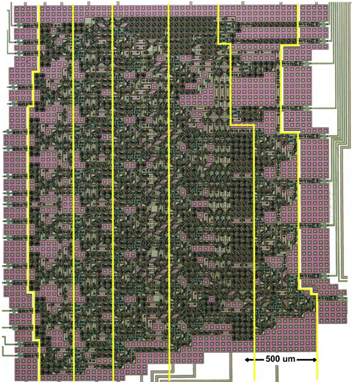
Figure 3.15 : 8-bit Kogge-Stone adder designed at TOBB ETU and fabricated by STP2 process [80].
