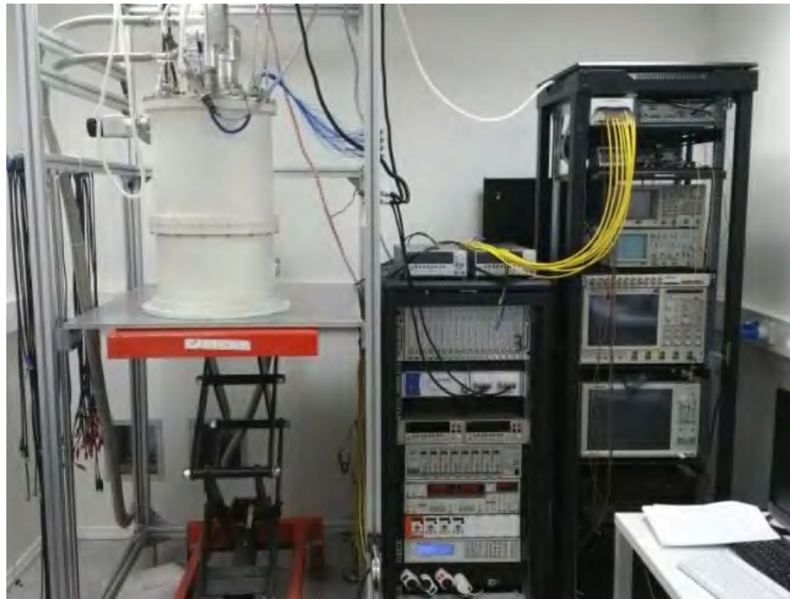
Figure 5.6 : The cryostat and the test setup for low and high frequency tests.
