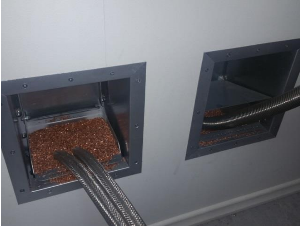
Figure 5.15 : The copper dust medium for insertion of the pipes.
